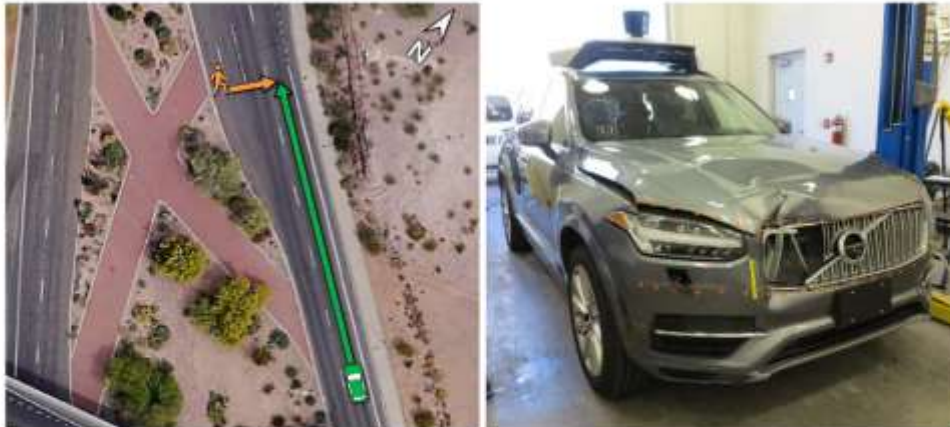
Figure 1. (Left) Location of the crash on northbound Mill Avenue, showing the paths of the pedestrian in orange and of the Uber test vehicle in green. (Right) Postcrash view of the Uber test vehicle, showing damage to the right front side.
